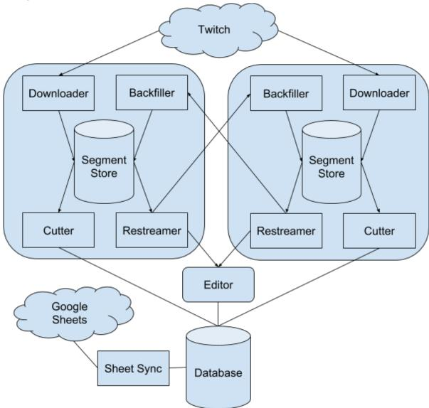
In the above, Editor runs inside a user's browser (though it wouldn't talk directly to the database, it would go via some simple api service, not pictured for clarity). The large encapsulating boxes represent an individual node. Sheet Sync and Database may run on one of these nodes, or elsewhere, it doesn't matter. Pictured is two nodes but you can scale out to any number. Additional nodes simply add more capacity to cut more videos at once, and greater redundancy.
